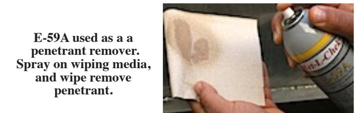
**E-59A used as a penetrant remover. Spray on wiping media, and wipe remove penetrant.**
