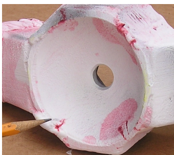
Visible penetrant indications of porosity on weld and stress cracks on metal clamp.
