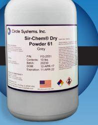
Sir-Chem<sup>®</sup> Dry Powder 61 is a highly refined nonfluorescent grey magnetic powder used for dry method magnetic particle inspection. It is designed to be used in visible light to reveal minute discontinuities on fabricated components or weldments such as bridges, pipes, large tanks, machinery and equipment.
