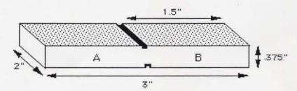
When comparing high temperature or low temperature penetrant performance to a standard penetrant at ambient temperature, it is essential to cut the panel into two separate sections. The section to be tested with high or low temperature penetrant will be heated or cooled, as appropriate, while the section to be tested with conventional penetrant remains at room temperature.
